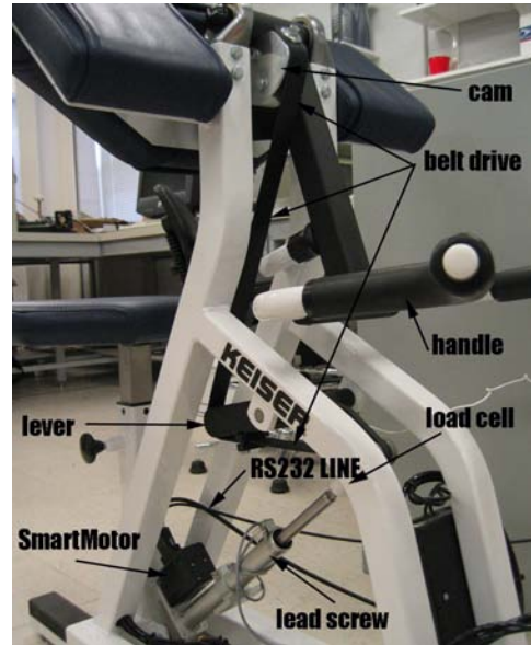
Fig. 2. View of arm curl machine showing the linear actuator connected to lever and belt drive.
