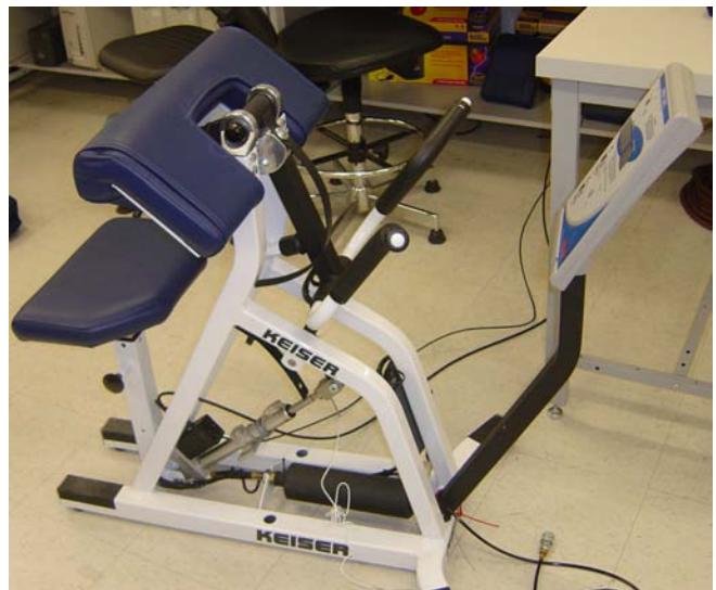
Fig. 1. Keiser Arm Curl 250 retrofitted with UltraMotion actuator.
