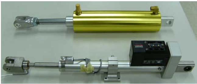
Fig. 7. Keiser pneumatic piston (top) versus Ultramotion lead screw actuator driven by SmartMotor (bottom).
