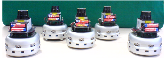
Fig. 1. A team of five Khepera robots. Each robot has an on-board Hokuyo range-finder and associated battery pack.
