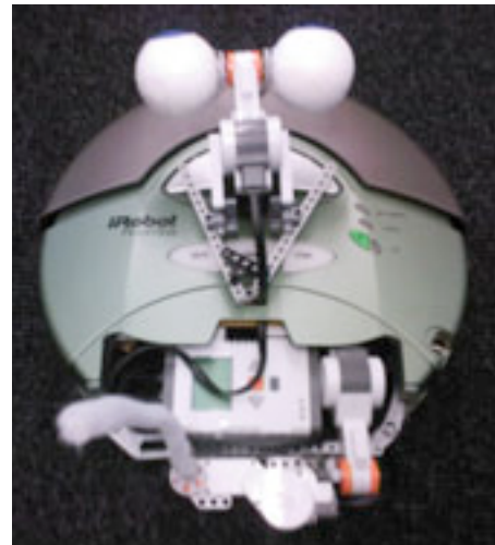
Fig. 3. Roomba with Lego NXT modification – rear hoover section removed and NXT brick in situ with three motors: tail mechanism and vertical eye movement.
