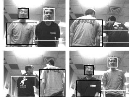
Fig. 4. Example person tracking scenario. In (a) and (b), our algorithm tracks persons with and without the primary characteristic (faces). After leaving the camera’s view, the two persons exchange their shirt, and re-enter the scene without showing their faces in (c). The algorithm classifies the persons by just the secondary characteristic. Once the primary characteristic is visible, it updates the secondary characteristic of each person in (d).
