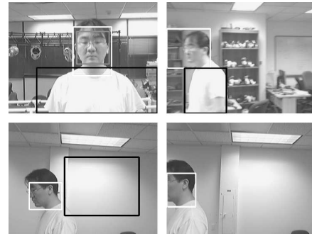
Fig. 6. Example person tracking scenario. Gray, white, and black bounding boxes are showing the primary characteristic (face), and the two secondary characteristics (face color and shirt color), respectively. In (a) and (b), our algorithm tracks a person with and without the primary characteristic, even in blurry images. The shirt color is not a good feature in a similarly colored environment like (c), but the face color classifier provides it with new negative samples, so that no false positives are returned (d).
