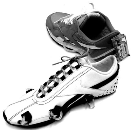
Fig. 6 Shoes with GCF measurement system: Air bladders and air pressure sensors are installed for measurement of ground contact forces.
