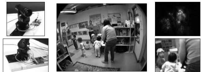
Fig. 4. Experimental Setup: A simple robotic camera (left) collected very wide angle – 160° – images at 640×480 resolution (center) and downsampled them to 160 × 120 resolution for the purpose of computing a saliency map (top right). The camera then rotated – pan/tilt – so that the maximum saliency pixel was now in the center of gaze. After movement, a 160 × 120 snapshot of the center of gaze at full resolution was saved as a foveal representation (bottom right). This fovea was coded offline for the presence of people.
