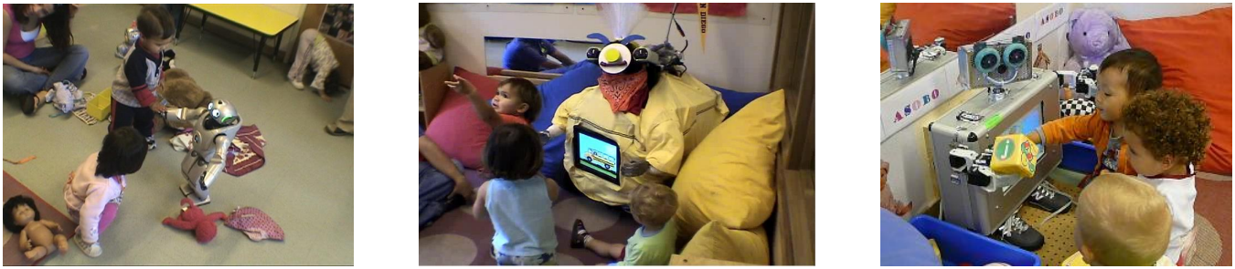
Fig. 3. Three robot members of the RUBI project. Left: QRIO is a humanoid robot prototype on loan from Sony corporation. Center: RUBI-1, the first prototype developed at UCSD. Right: RUBI-3 (Asobo) the third prototype developed at UCSD. It teaches children autonomously for weeks at a time
