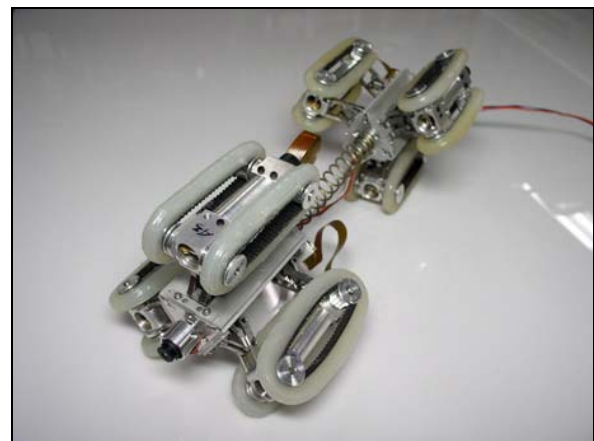
Fig. 1. Whole view of the pipeline inspection robot
