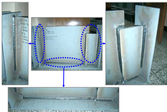
Fig. 18. Test results of the movement in the transverse direction of 'Rail Runner'
