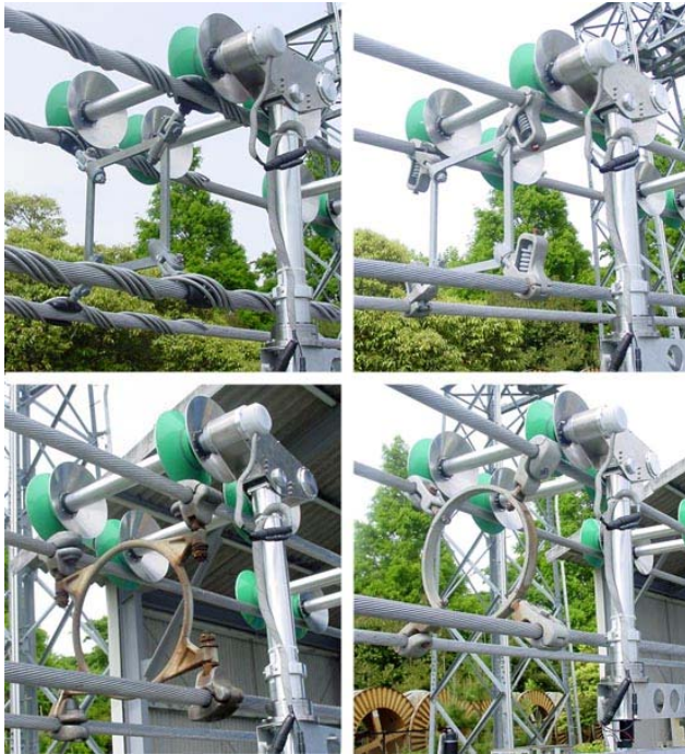
Fig. 9. Motion unit of Expliner overcoming four different cable spacers
