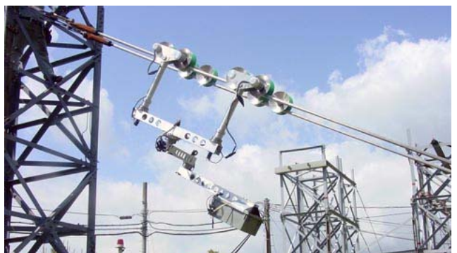
Fig. 12. Expliner moving on inclined cables (inclination: 30 degrees)
