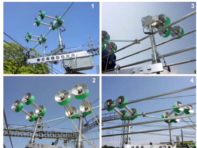
Fig. 11. Sequence of pictures of Acrobatic Mode 2 (1: moving on access cable; 2: lifting front motion unit; 3: aligning front motion unit with power lines; 4: placing front motion unit on power lines)
