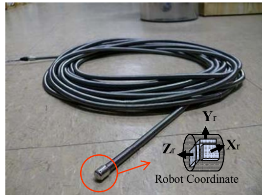
Fig. 13. Construction of 3 single-axis gyro sensor
