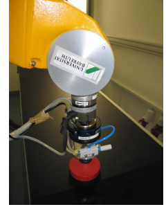
Figure 3: Setup of the second experiment. The vacuum gripper grasps the disk at specified offsets from the center and measures the forces and torques for each position. Based on this information the drift compensation function is approximated using a Householder approximation and a MLP neural network.
