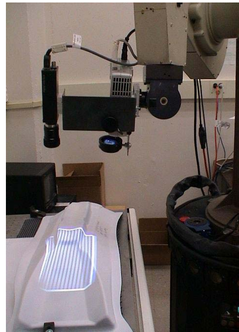
Fig. 8. A robot-aided 3D dimensional inspection system
