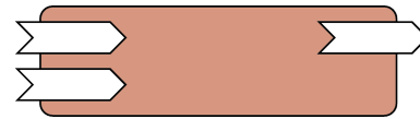
Fig. 13. Example for a component of the programming environment with two input and one output ports.
