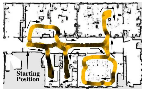
Fig. 2. Traditional sensor models which ignore the multi-modality in the distribution of beam lengths become inaccurate in the proximity of doors, corners, and clutter. In this diagram, dark parts of the trajectory mark locations, where the true pose receives a high likelihood relative to neighboring ones, while orange/brightly colored parts highlight the less accurately modeled locations.
