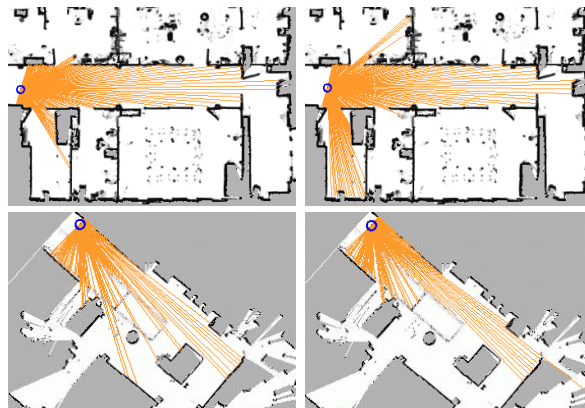
Fig. 1. In mobile robot localization, small variations in the robot pose can cause large changes of the range measurements. This leads to multi-modal distributions of beam-lengths in the local neighborhood of a pose hypothesis.
