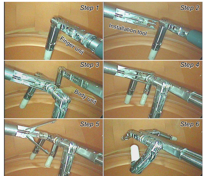
Fig. 15. Assembling experiment in a closed space
