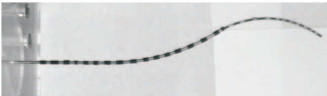
Fig. 8. Experimental photo from one of the stereo cameras showing the cannula with fiducial markers.
