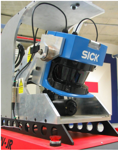
Fig. 1. The nodding 3D laser range finder mounted on a mobile robot
