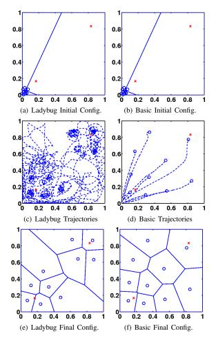
Fig. 6. The initial configuration, robot trajectories, and final configuration are shown for a network of robots with the adaptive ladybug controller on the left (6(a), 6(c), and 6(e)) and with the basic adaptive controller on the right (6(b), 6(d), and 6(f)). The Gaussian centers of  $\phi(q)$  are marked by the red x's.
