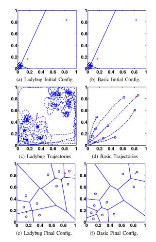
Fig. 3. The initial configuration, robot trajectories, and final configuration are shown for a network of robots with the non-adaptive ladybug controller on the left (3(a), 3(c), and 3(e)) and with the basic non-adaptive controller on the right (3(b), 3(d), and 3(f)). The Gaussian centers of  $\phi(q)$  are marked by the red  $\times$ s.
