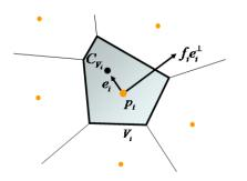
Fig. 2. A geometric representation of the non-adaptive ladybug controller is shown. The robot is at  $p_i$ , its Voronoi region is labelled  $V_i$ , with a centroid at  $C_{V_i}$ . The two components of the control law are shown as perpendicular vectors,  $e_i$ , the coverage force, and,  $f_i e_i^{\perp}$ , the exploration force.
