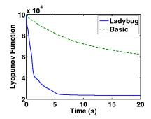
Fig. 5. The decreasing Lyapunov function is shown for both the ladybug and the basic non-adaptive controllers. The ladybug controller achieves a lower value.
