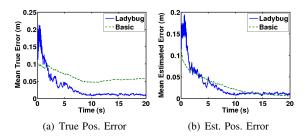
Fig. 7. The true position error  $e_i$  is shown on the left and the estimated position error  $\hat{e}_i$  on the right averaged over all of the robots for the ladybug and the basic adaptive controllers. The convergence of  $\hat{e}_i$  is guaranteed by Theorem 2 for both controllers, however the ladybug controller leads to a lower true position error.
