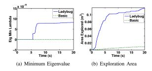
Fig. 9. The left plot shows a metric indicating the richness of the robot trajectories. A larger value denotes faster parameter convergence and also indicates more exploration. The ladybug controller gives richer trajectories than the basic controller. The plot on the right shows the minimum over all the robots of the area explored during a trajectory. Again, the ladybug controller causes the robots to explore more of the space than the basic one.
