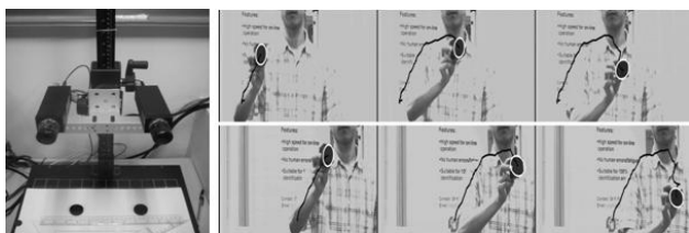
Fig. 6. The stereo setup and snaps of the stereo trajectory tracking
