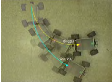
Fig. 8 Calibration Experiments for steering angles for only two steering inputs when \phi=12.4^\circ, 20.4^\circ
