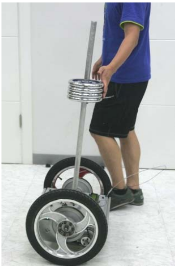
Figure 7. The pendulum coordinating with an external force applied by a human
