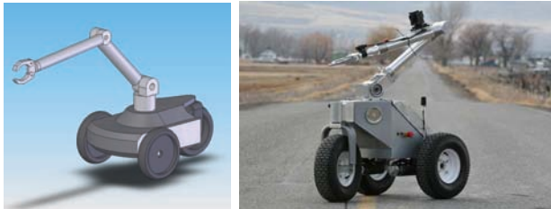
Fig. 1. Early Concept and Final Prototype of the UGV Modeled in This Paper.
