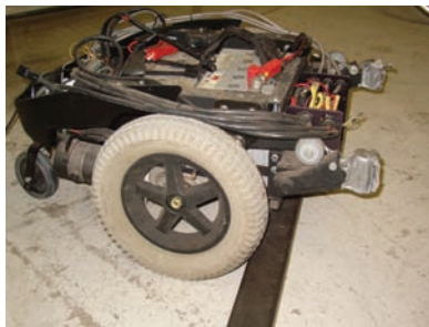
Fig. 14. Wheelchair Wheel Friction Measurement (top) and Wheelchair Against Step (bottom).
