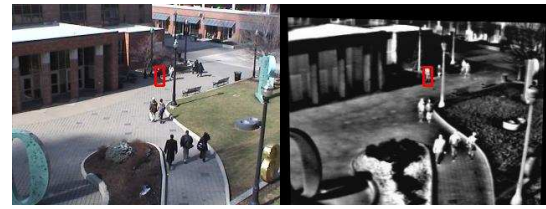
Fig. 3. The approach “Infrared”. Left: Frame 511; Right: Frame 564. (Note that the passing person walks to the left and the true object walks to the right. The tracker locks onto the passing person and the tracking totally fails.)
