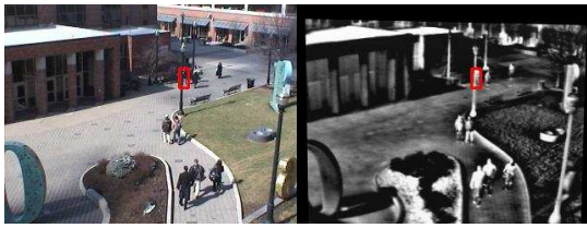
Fig. 3. The approach “Infrared”. Left: Frame 511; Right: Frame 564. (Note that the passing person walks to the left and the true object walks to the right. The tracker locks onto the passing person and the tracking totally fails.)
