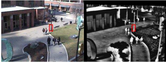
Fig. 4. The approach “Average”. Left: Frame 601; Right: 691. (After the object leaves the telegraph pole and re-appears, the tracking results never recover.)
