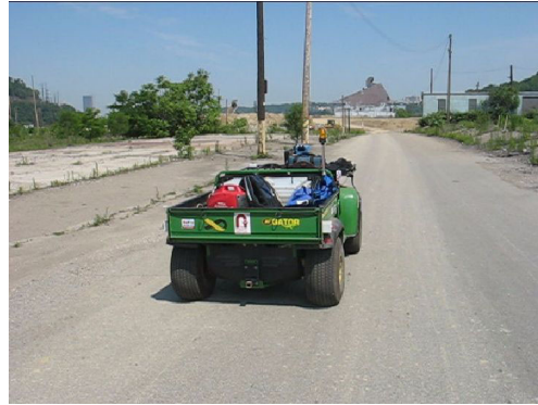
Fig 8. E-gator autonomous vehicle used for testing and electric poles used for localization at test site. The vehicle equipped with wheel encoders and a KVH E-core 1000 fiber-optic gyro for dead reckoning, and a tilting SICK lidar and onboard computing for navigation and obstacle detection
