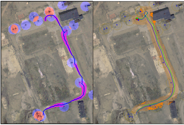
Fig 9. Path planned (left) and executed (right) without GPS using RPUP. In the left image the blue circles are unique detection regions generated by landmarks. In the right image, the blue line is the position estimate of the Kalman filter on the robot and the green line is the position reported by a WAAS differential GPS with accuracy of approximately 2 meters (for reference only). The orange regions represent sensor data, with obstacles shown as bright orange.
