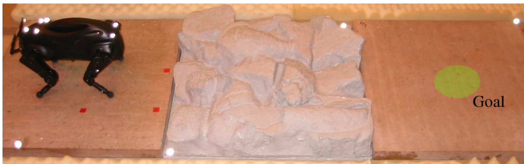
Fig. 6. Example of a typical setup for the robot and terrain (shown here with Terrain #3).
