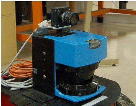
Fig. 3. The camera and the laser range sensor used in the experiments.
