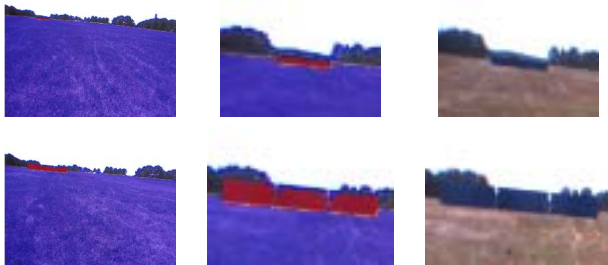
Fig. 3. The long-range classified image (left column) showing traversable (blue) and non-traversable (red) terrain, a zoomed in view of the classification (center column) and original image (right column) at 100m (top row) and 30m (bottom row)
