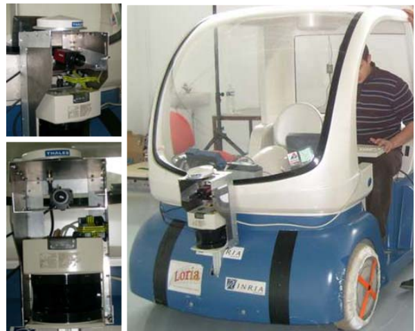
Fig.3: Sensors embedded on the vehicle
