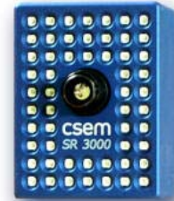
Fig. 1. Photo of the SR-3000 3D Camera
