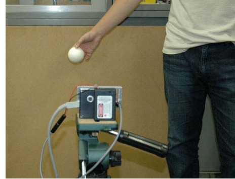
Fig. 14. Scene of measuring a falling ball with the constructed sensor
