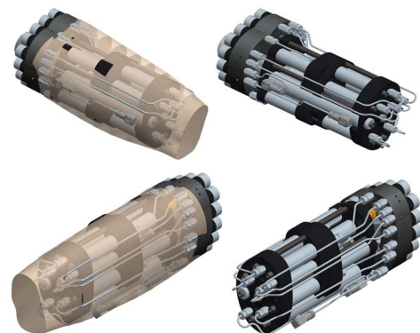
Fig. 2. (left) Solid model of the forearm actuation unit within the volume constraint of a fifty percentile female volume. (right) Solid model of the actuation unit.
