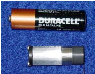
Fig. 4. Stand-alone miniature servovalve, shown next to a AA-sized battery.
