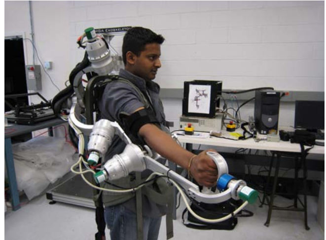
Fig. 1. The MGA Exoskeleton has five powered joints including a three-axis intersecting shoulder and a scapula elevation joint.
