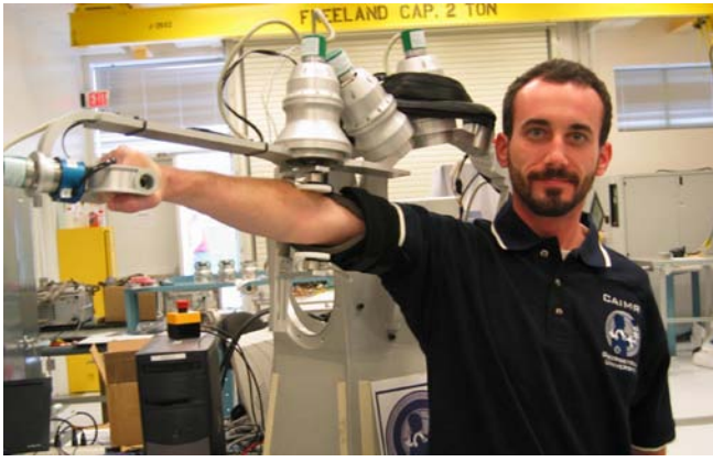
Fig. 6. Exoskeleton shown at 90° shoulder abduction.
