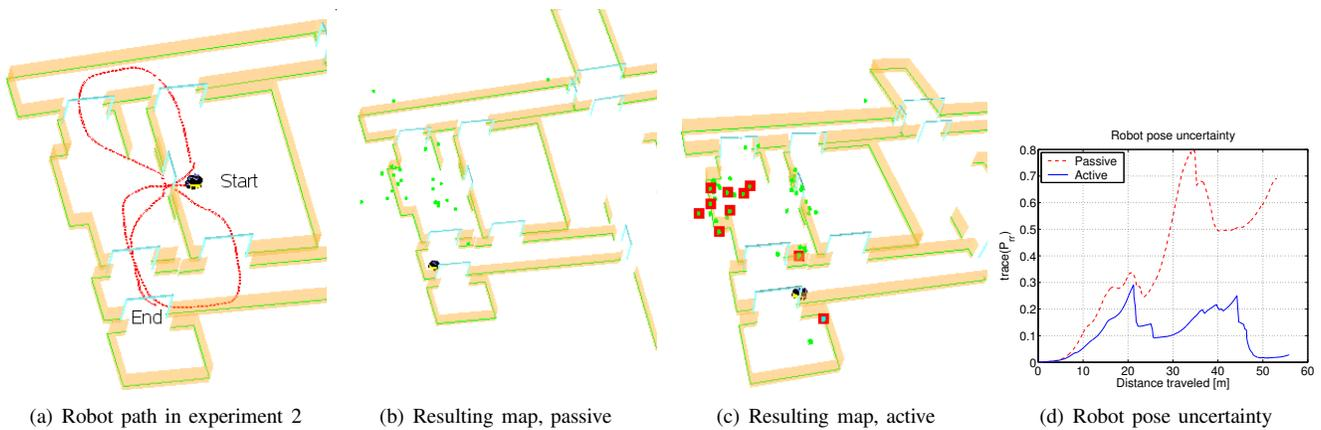
Fig. 6. Experiment 2: comparison of passive and active camera control. Green, small dots are landmarks (b,c), red, large dots are database matches (c). (d): the robot pose uncertainty computed as the trace of  $P_{rr}$  (covariance of robot pose) for passive and active camera mode. A video showing the trajectory of the robot in active camera mode is available on the CD proceedings of ICRA 2008.
