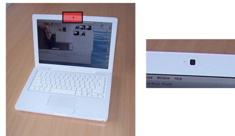
Fig. 3. Built-in iSight video camera on an Apple Macbook . This camera was the sole source of sensory information for all experiments. The laptop was mounted on the roof of a car in a forward facing, neutral pitch position.
