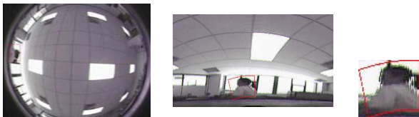
Fig. 2. An omnidirectional image, its corresponding panoramic image and the pattern of the detected object
