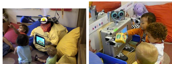
Fig. 1. Two of the robots developed as part the RUBI project. Top: RUBI-1, the first prototype was for the most part remote controlled. Bottom: RUBI-3 (Asobo) the third prototype teaches children autonomously for weeks at a time
