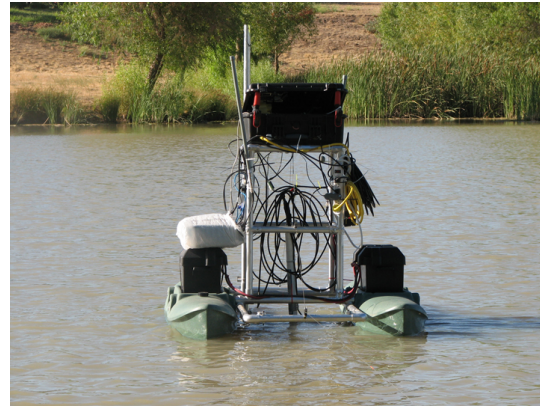
Fig. 1. Aquatic Networked InfoMechanical System (NIMS AQ).
