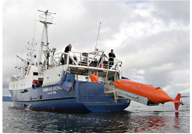
Fig. 4. The HUGIN 4500 AUV prior to sea-trial launch in October 2006.
