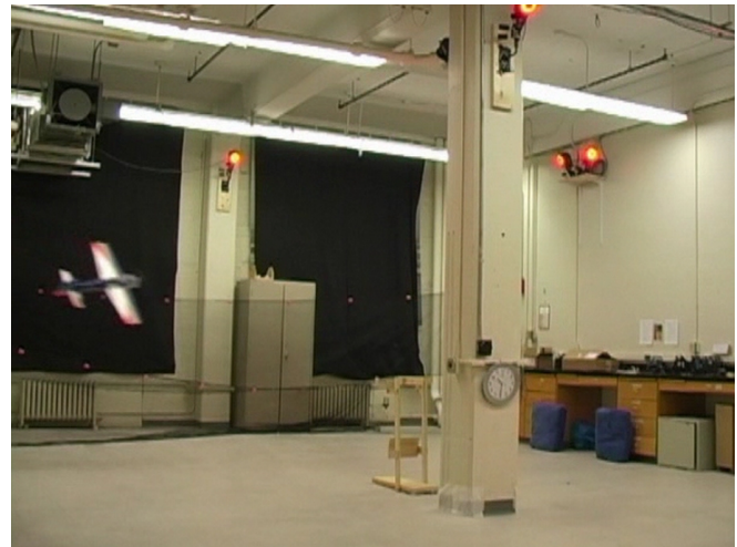
Fig. 3: Aircraft performing a three-lap maneuver after transitioning from hover flight.
