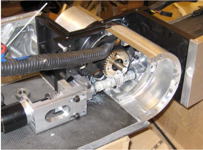
Figure 3: The inner workings of the passive compliant body joint. The worm is cushioned on the axle by Bellville springs. The wiring pass through can be seen above the driven worm gear.
