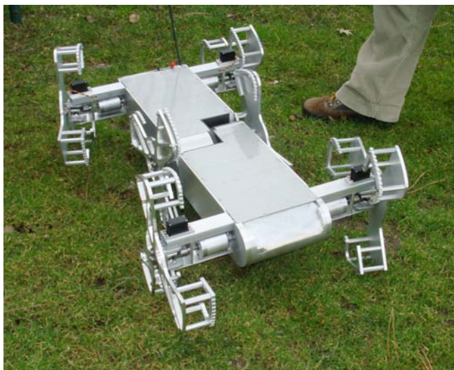
Figure 1: DAGSI Whegs™ with outdoor feet.
