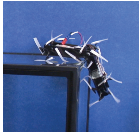
Fig. 1. Climbing Mini-Whegs™ using a body joint
