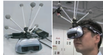
Fig. 2. Video See-Through HMD: VH2002 with Marker Balls
