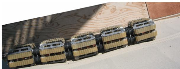
**Figure 2:** Our earlier-developed and larger OmniTread OT-8 can fit through an 8-inch diameter hole. Here it is driving up an inclined sand pit.
