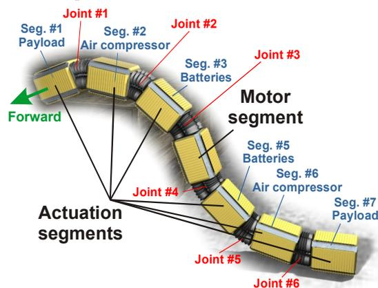
**Figure 3:** The OmniTread Model OT-4: Nomenclature for segments and joints.
