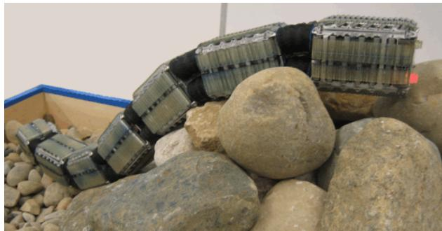
**Figure 1:** The OmniTread OT-4 serpentine robot climbing over a pile of rocks.
