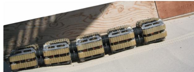
**Figure 2:** Our earlier-developed and larger OmniTread OT-8 can fit through an 8-inch diameter hole. Here it is driving up an inclined sand pit.
