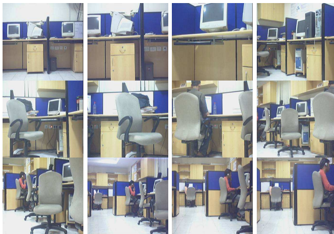
Fig. 9. Navigation Result: The sequence of images (seen from the robots view) while servoing from start pose (top left) to the goal pose (bottom right).
