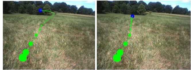
Fig. 9. Example of the effect of pitch error on goal point projection and the image-based planned path.
