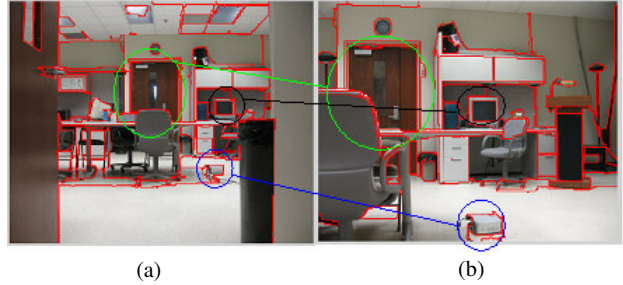
Fig. 4. Loop detection in an indoor environment: (a) was the image taken close to the point of loop-closure (b) was the image taken at the starting point. About 10 pair of objects got matched. The green, blue and black circles show three pairs of the matched objects.
