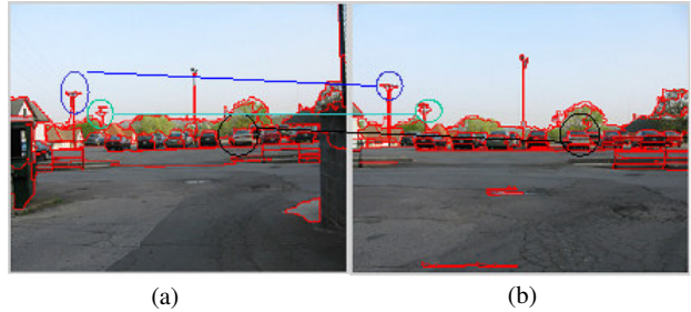
Fig. 5. Loop detection in an outdoor environment: (a) was the image taken close to the point of loop-closure (b) was the image taken at the starting point. About 12 pair of objects got matched. The green, blue and black circles show three pairs of the matched objects.
