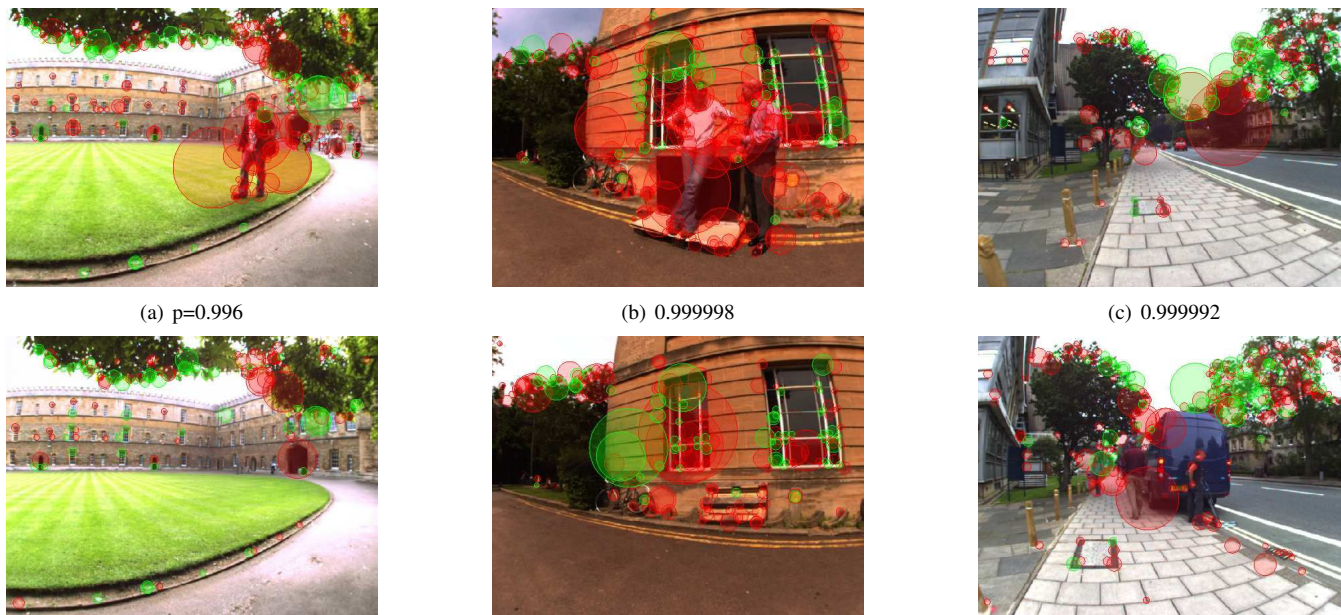
Fig. 6. Some examples of images that were assigned high probability of having come from the same place, despite scene change. Results were generated using the accelerated likelihood calculation. Words common to both images are shown in green, others in red. The probability that the two images come from the same place is indicated between the pairs.
