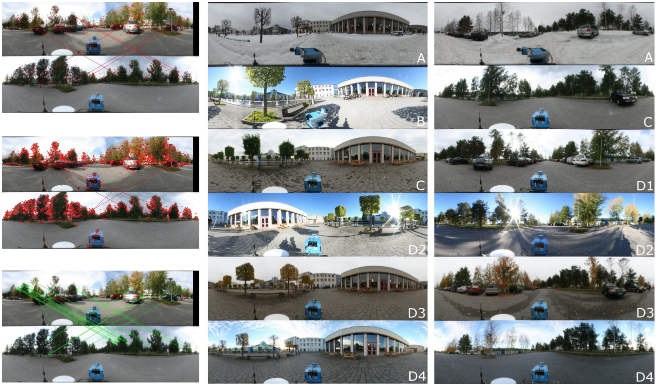
Fig. 2. Left, top: Low-resolution panoramic images matched using U-SURF, relative threshold of 0.65. Left, center: High-resolution panoramic images matched using U-SURF, relative threshold of 0.65. Left, bottom: High-resolution panoramic images matched using U-SURF, relative threshold of 0.80, reciprocal matching. Epipolar constraint applied. Center: Images from northwest part of map. Right: Images from parking lot to the south.
