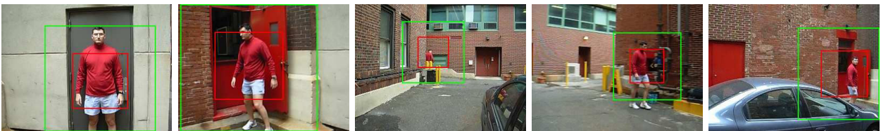
Fig. 4. ABCshift successfully tracks throughout the sequence and is not distracted by red regions of background, despite being initialised in image 1 which contains no red background. Frames 1, 176, 735, 1631, and 1862 shown. Green and red squares indicate the search window and estimated object size respectively. This movie, PeopleTracking1ABCshift.avi, can be viewed at our website[19].
