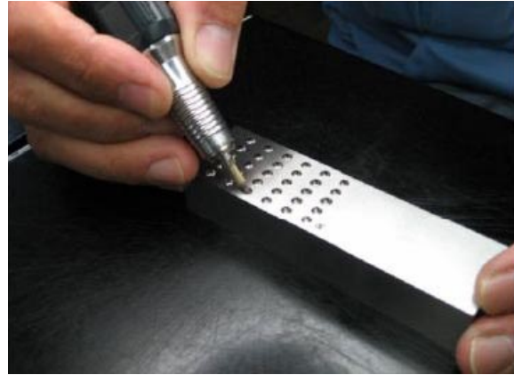
Fig. 1. Hand lapping scene of an LED lens mold.
