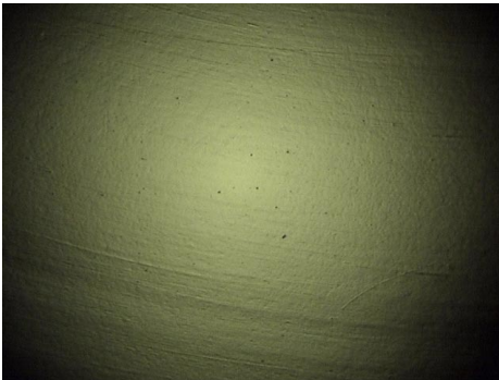
Fig. 13. Large scale photo of the LED lens mold after the lapping process by using the proposed stick-slip motion control.
